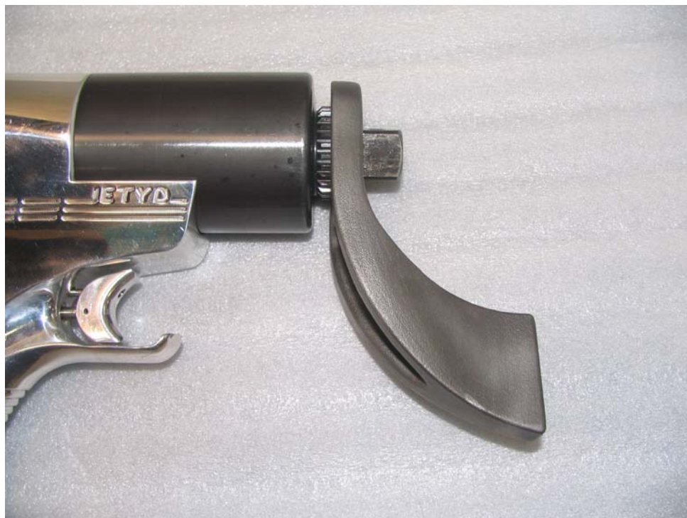
Figure 4. Reaction Arm Installed
