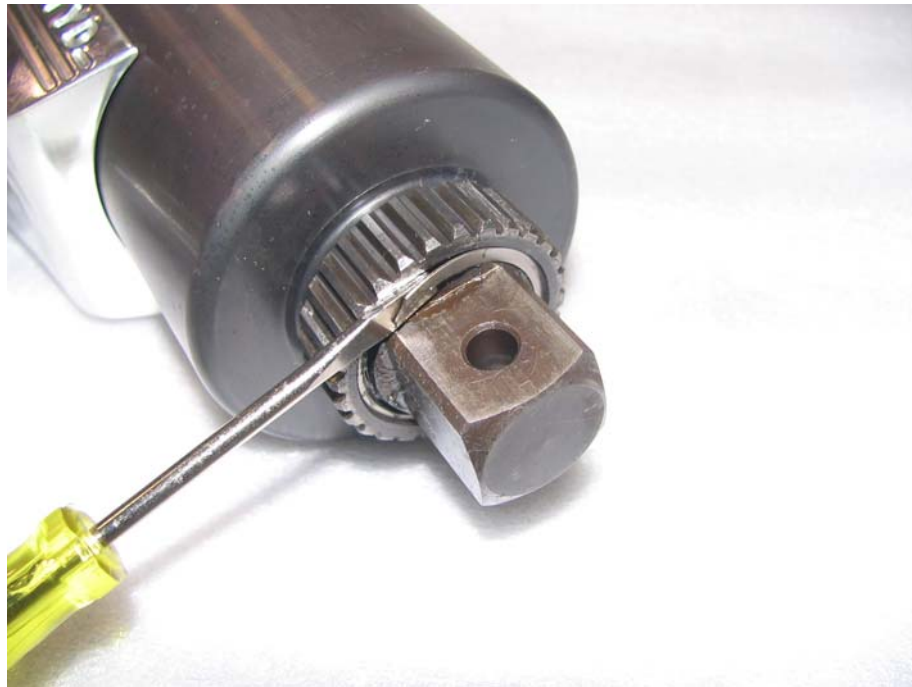
Figure 12. Removing the jGun Square Drive Snap Ring
