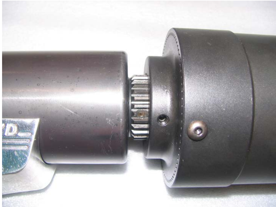
Figure 25. Aligning LoadDisc Socket Set Screw with Machined Recess in jGun Splines
