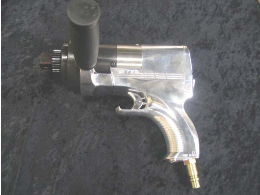
Figure 13. Dual Speed jGun with Handle
