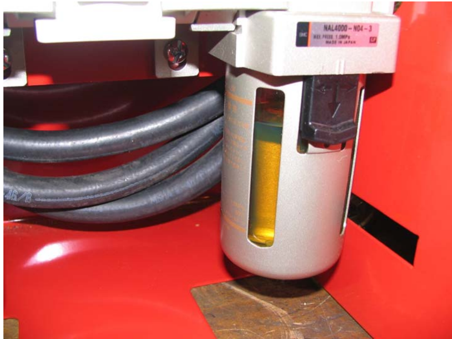
Figure 19. FRL Unit – Lubricator 2/3rds Full of Oil
