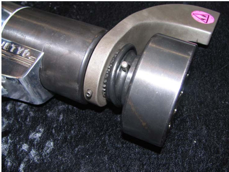
Figure 7. Installing Socket Locking Pin and Retaining Ring
