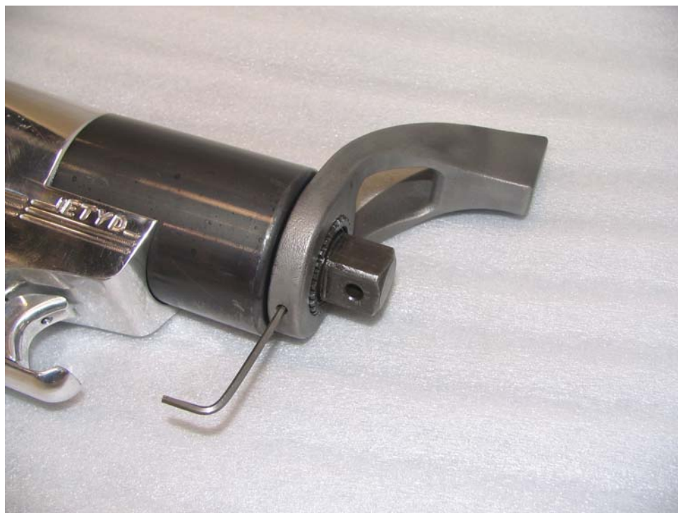
Figure 5. Tightening Reaction Arm Set Screw
